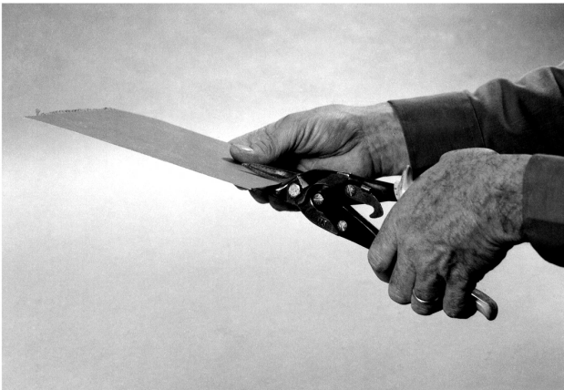
FIGURE 4.27 Wrist angles during tool use
