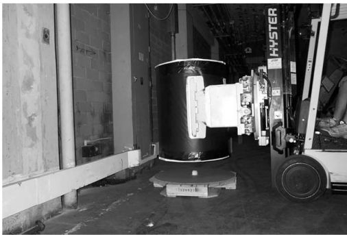
Fork Truck with Drum Handling Attachment
