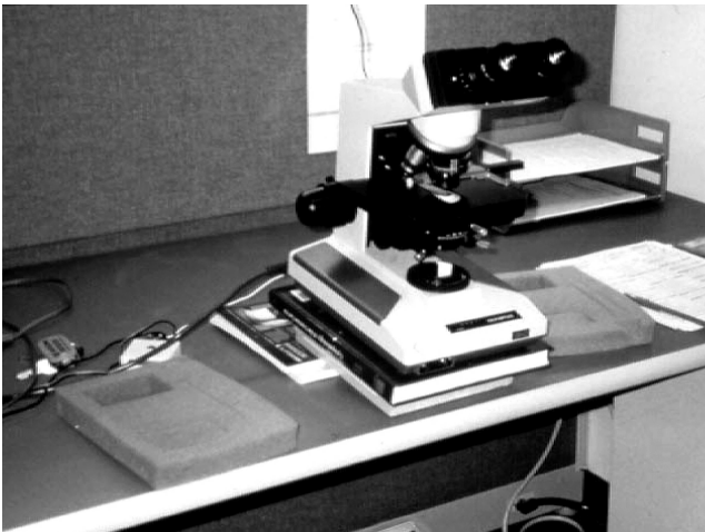
FIGURE 3.16 A microscope adjusted for height and angle by using books. Foam pads are present on either side to cushion the elbows.
