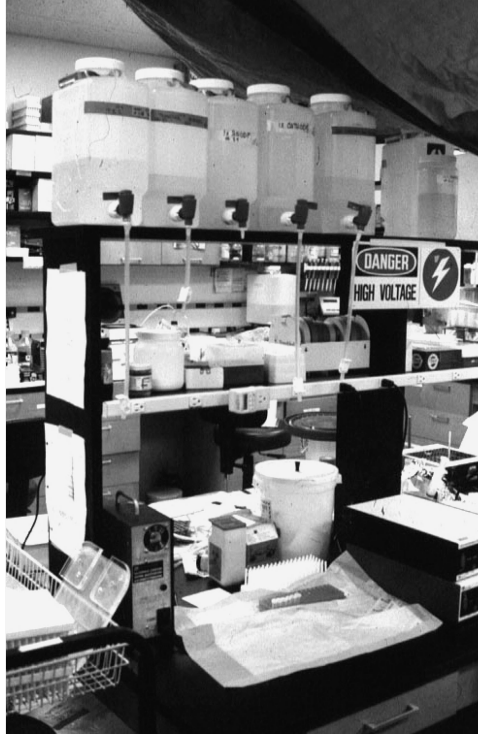
FIGURE 7.12 An example of an organized laboratory bench with large bottle dispensers on the top shelf. The location is convenient for use but creates a manual material handling concern to place full bottles on the shelf.
