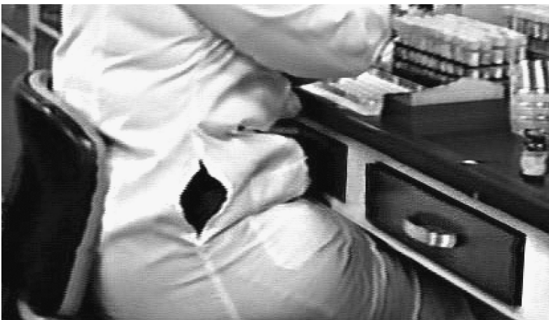
FIGURE 3.14 An illustration of the lack of thigh clearance when sitting at a bench that has drawers along the top edge of the leg well
