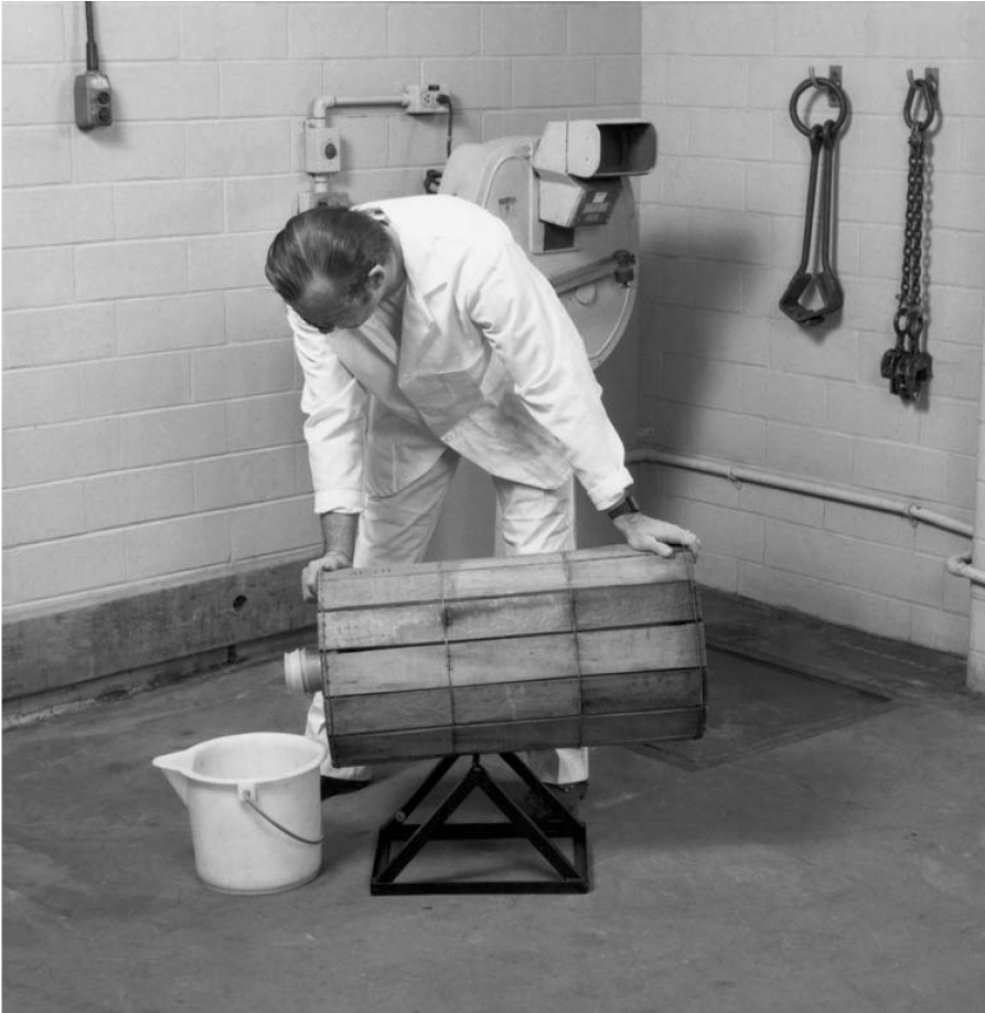
FIGURE 7.11 A tipping stand to control flow from a carboy
