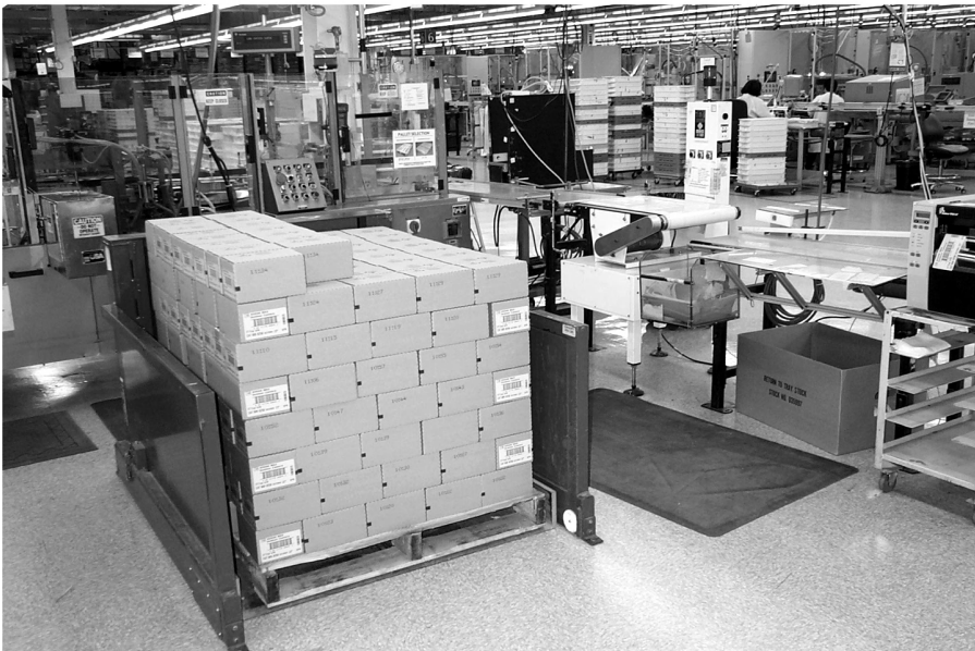
FIGURE 3.38 Lift Table for Adjusting the Height of a Pallet
